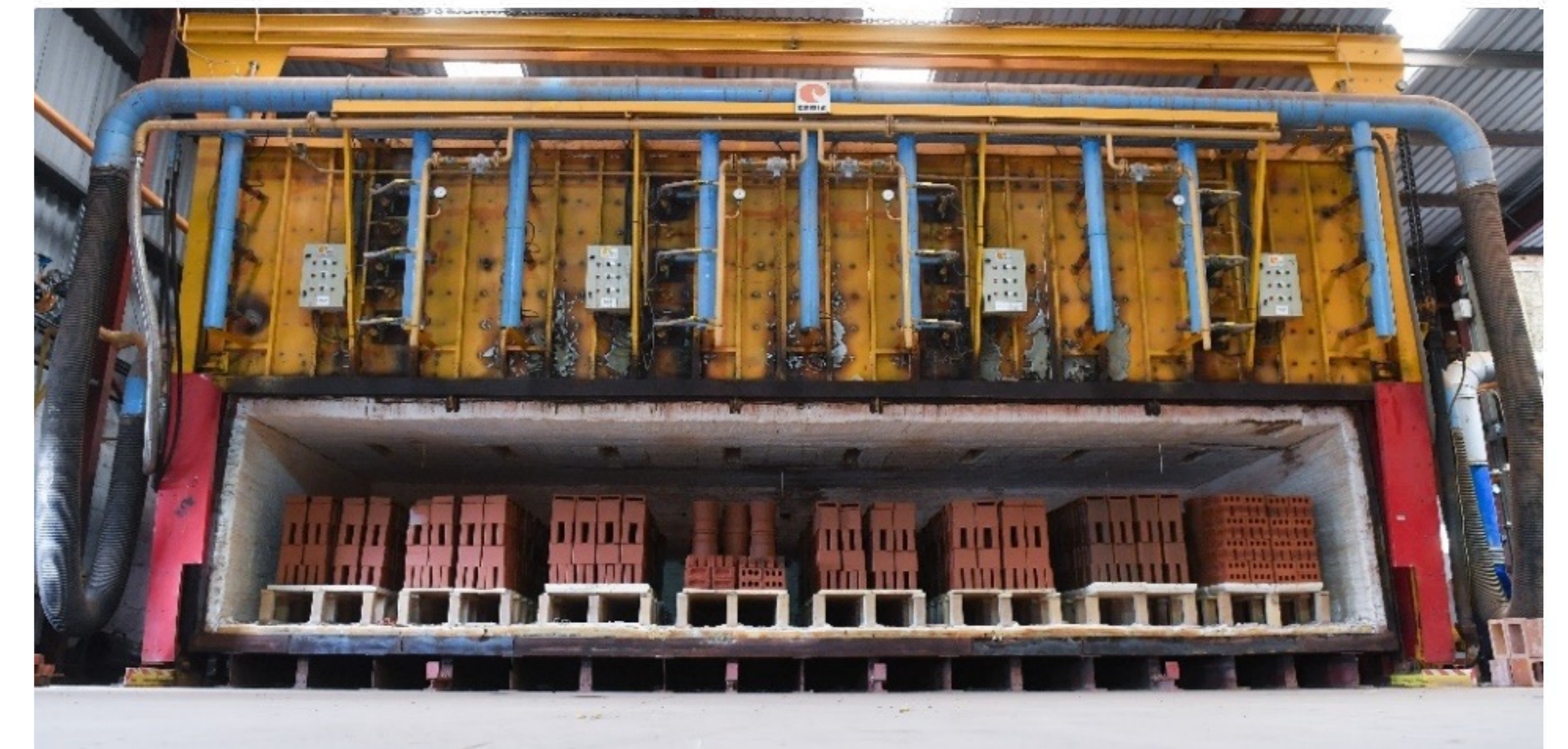
Credit: Forterra Plc - Hydrogen firing trials
