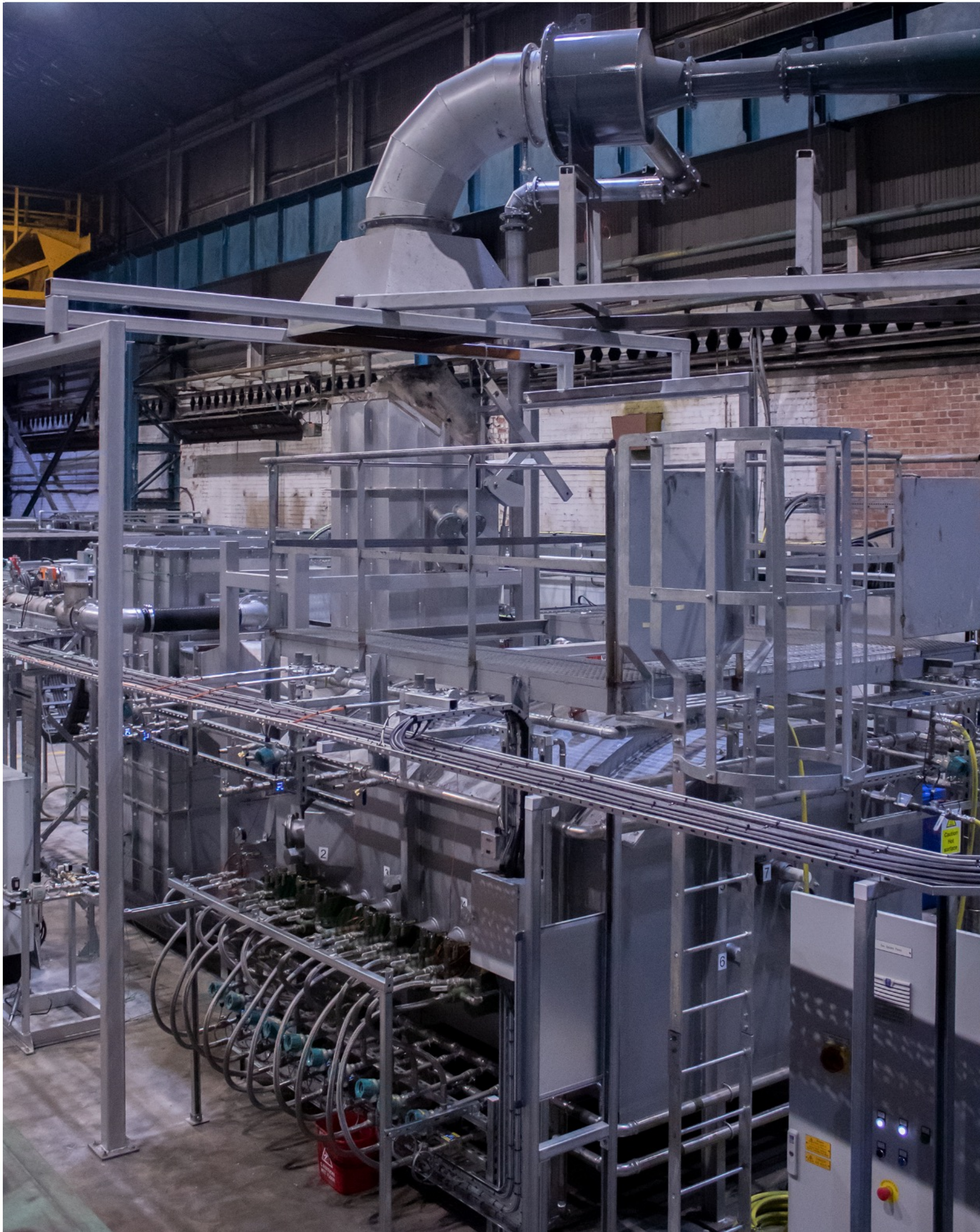
Credit: Glass Futures' Hydrogen test bed rig - Phase 1 'Hydrogen for the Ceramic Sector' research project
